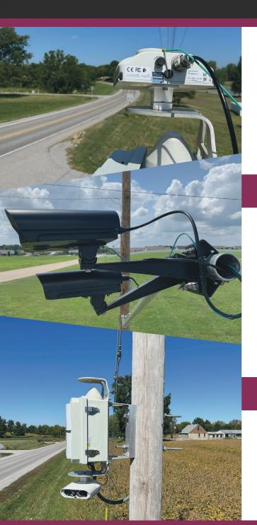
Utilitra's custom network enclosures are designed to provide a custom installation for situational cameras (fixed or pan-tilt-zoom) and/or license plate recognition cameras. The enclosures are NEMA rated IP66 allowing the deployment of the network enclosures in any environment. The Utilitra network enclosures are lightning protected and contain a PoE switch as well as a push button to remote reboot the enclosure.
